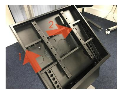
Remove the two arms from the bracket and mount these to your screen using the four M8 screws provided. If these are not appropriate for your screen please use the correct screws to fix the arms to your screen.
