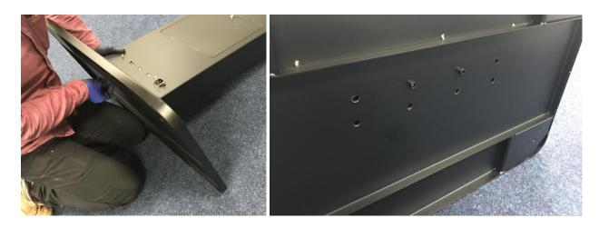
**Step 2**Screw the remaining six M8 hexagon socket head bolts in by hand then tighten all eight up with a size 6 hex key.
