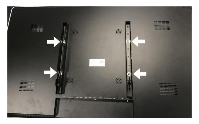
Attach the bracket back onto the arms and fix the arms to the bracket by screwing in the hexagon socket head bolts attached using a size 5 hex key.
