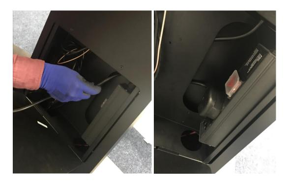
Connect the ends of extension cables, including the power cable, to the inputs of your screen.
